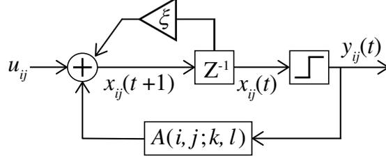
Fig. 5: The block diagram of a cell of the SD-CNN
